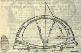
Fig. 19.—Reinforced Concrete Sewer.
